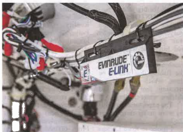
The E-Link dongle connects to the data backbone of the outboard network and can sit out of sight. The app is free.
