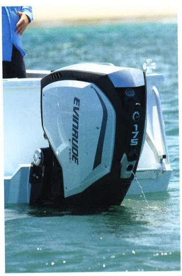
Also part of the new series is what Evinrude calls I-Trim, It's standard on all Gen 2 models and assists the boat driver with automatic engine trim adjustment according to speed. There are five I-Trim profiles available for selection, and all the operator has to do is choose the profile that best suits the conditions of the day, and the engine will adjust its trim angle automatically. This can be manually over-ridden at the touch of the trim button, much like an automotive cruise control system.
